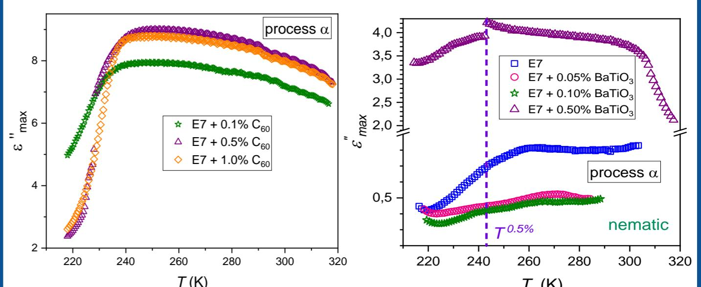
Temperature evolutions of  $\alpha$  process primary loss curve maximum in the nematic phase of E7 and related nanocolloids with BaTiO<sub>3</sub> and C<sub>60</sub> nanoparticles. On the right chart the discontinuous change emerges for 0.5 wt. % BaTiO<sub>3</sub>. The loss curve peak  $\epsilon''_{\text{peak}}(T)$  shapes strongly depend on NPs types and concentrations.
