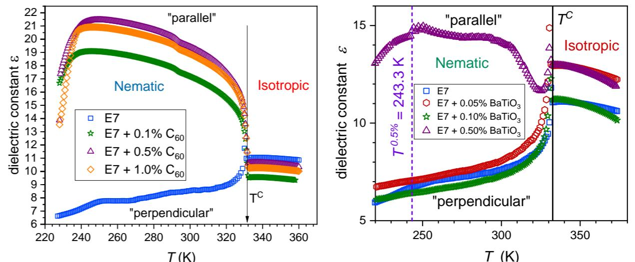
The solid arrow indicates the clearing temperature at  $T^C = 332.9$  K, related to weakly discontinuous I-N phase transition. 'Parallel' and 'Perpendicular' denote dielectric responses resembling those of nematic samples with the probing electric field oriented parallel or perpendicular to the long molecular axis, respectively. Introducing even a small concentration of C<sub>60</sub> results in a shift of the preferred alignment toward the parallel-like response.
