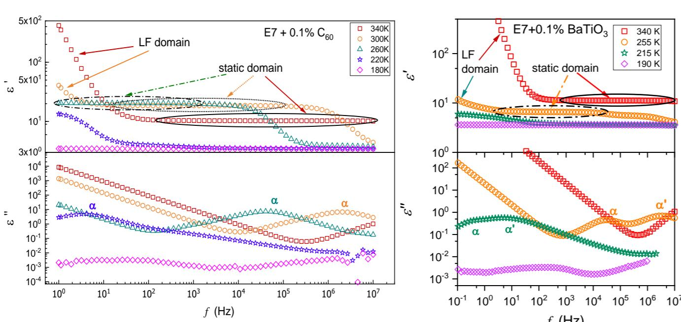
The real part of dielectric permittivity ( $\epsilon'$ ) exhibits a pronounced temperature dependence in static domain. In the imaginary part of dielectric permittivity ( $\epsilon''$ ), a clear temperature induced shift of the  $\alpha$ -relaxation is observed. With addition of 0.1 wt. % C<sub>60</sub>  $\alpha'$ -relaxation disappears.
