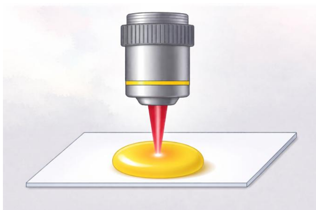
Figure 3: DLW via 2PP, enabling localized 3D fabrication within a photoresist.
